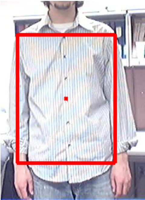
Fig. 2. An example training image used for both vision trackers: the kernel-based object tracking (in KernelObjTracker ) and the motion-focused color histogram correlation (in ColorHistTracker ). The trackers use the image region bounded by the red rectangle to initialize their target models. The red dot marks the center of the rectangle. Note that in the kernel-based method, the target model uses points in an ellipse with axis end-points at the mid-points of the rectangle sides, as opposed to all pixels in the bounding rectangle. The rectangle (i.e., the bounding region used for the target model) has size 162 \times 212 pixels. The fixed kernel bandwidth h = 0.6 .
