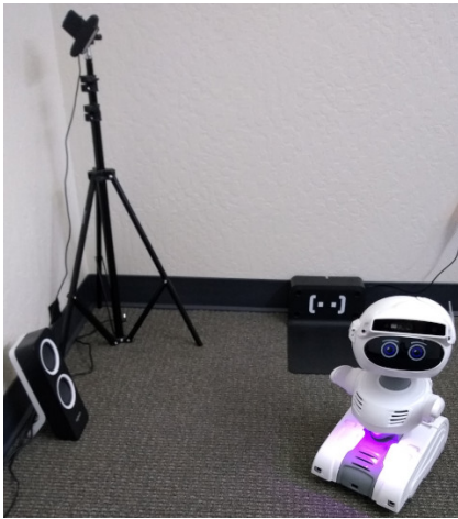
Fig. 3. Misty and the experimental environment, including speaker, overhead camera, and charging pad, as described in Section IV-A.
